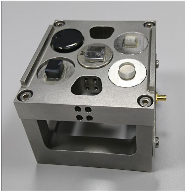
Default sample holder of the ZHN for five samples. It has an isolated surface and a connector for resistance measurements between (conductive) tip and sample
