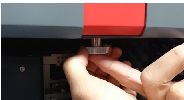
Tool for changing tips without additional protective measures
